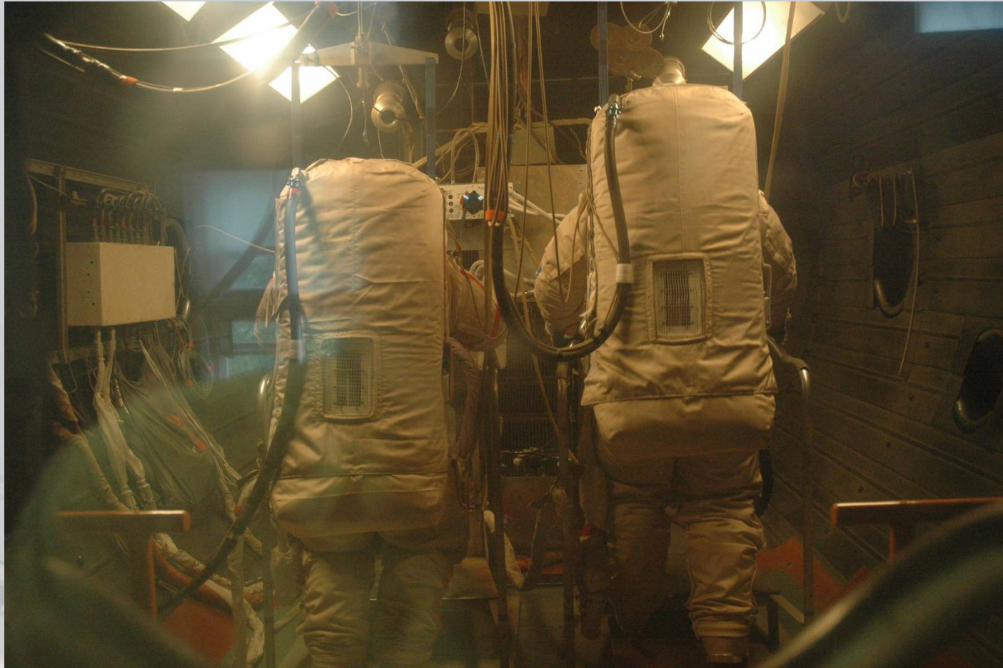
Taikonauts carrying out low-pressure training in extravehicular spacesuit test module
